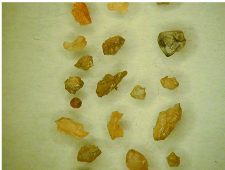
Figure 2. Example of 2,4,6-trinitrotolune (TNT) particulates found in military impact areas from a low-order detonation.
