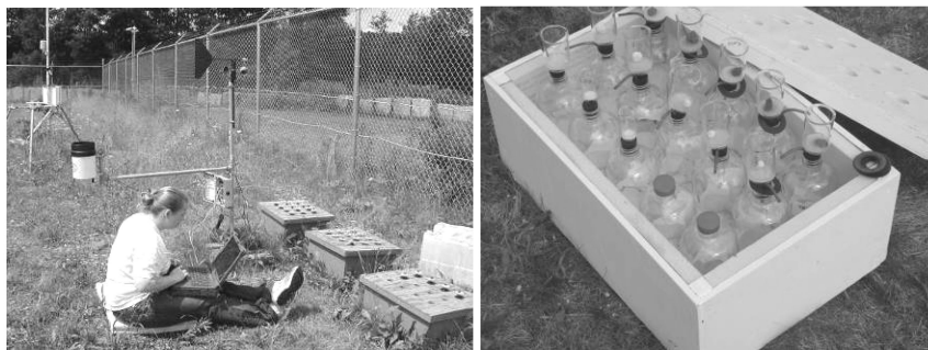
Figure 5. Outdoor tests showing Buchner funnels used to hold the HE pieces. Any precipitation landing in the funnel moves through the glass frit and into 1-L glass bottles in the wooden boxes.
