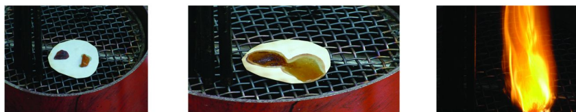
Figure 2. (Left) Initial melting, (Middle) Liquid state, (Right) Combustion. (see color insert)
