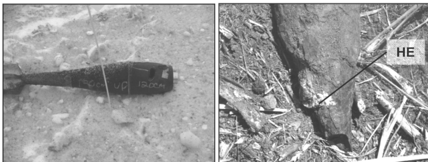
a. 81-mm round pierced by a fragment from a high-order detonation b. Exposed HE on a corroded 60-mm UXO
